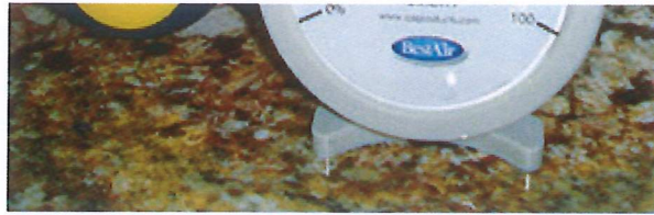
Just using a hygrometer is not enough-you need to make sure it's correct. Here a hygrometer that was left on the job site shows a substantially different reading than the properly calibrated hygrometer on the left. (Photo courtesy of Roy Reichow)
