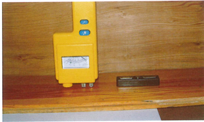
A pin meter is inserted in flooring ready to take a reading; note that a reference standard to check accuracy of the meter readings is shown on the right.
