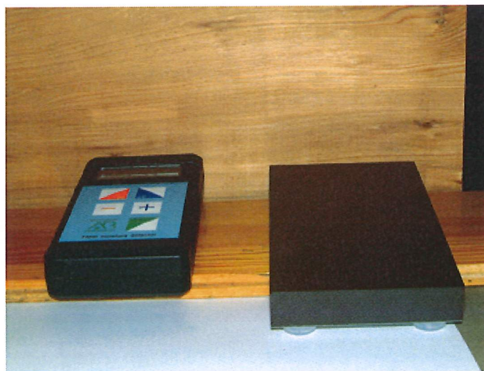
This pinless meter is shown with a calibration block that verifies the meter is working correctly on the right. The preferred direction with this moisture meter model is across the grain.
